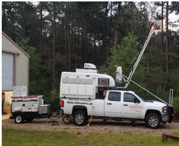
Figure 1. Photograph of the MAQL with arm raised and an available generator.
